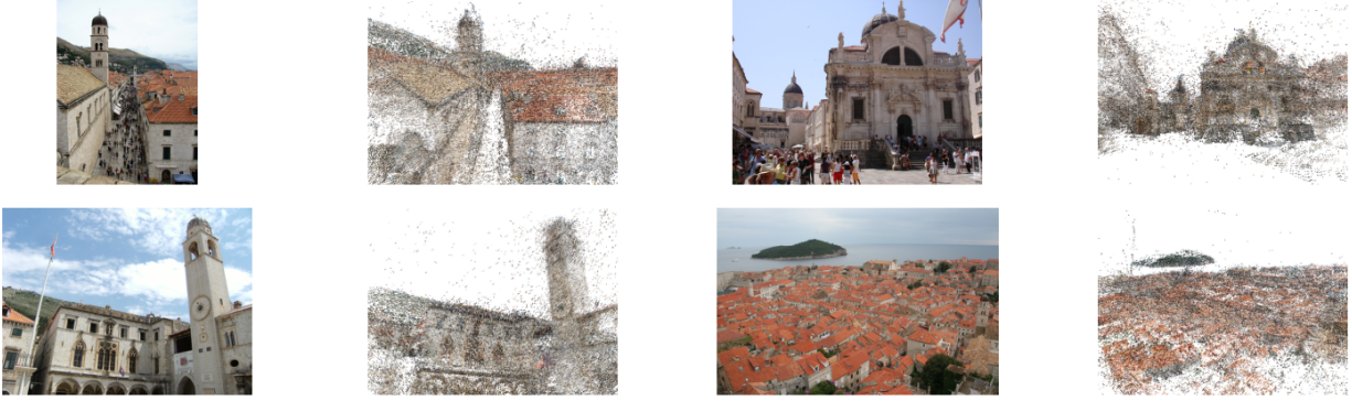
Figure 7: Four different views of the city of Dubrovnik with the corresponding view of the reconstruction. This reconstruction consisted of 4,585 images and 2,662,981 3D points with 11,839,682 observed features. Figure courtesy of [2].
